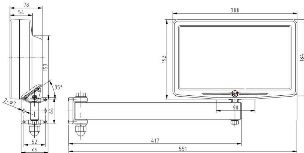
SUPPORTO CON PROLUNGA SDS6 PER MACCHINE TIPO FRESA
